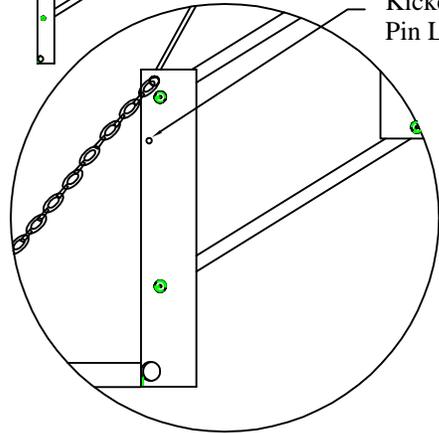
Step 2A. If the Liftgate had kicker springs previously installed in the upright fronts, grind off head on the kicker spring pin, then remove the pin and kicker spring. When grinding, wear some type of eye protection.
