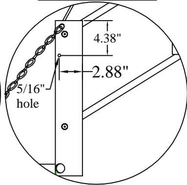
Step 3. Insert kicker spring inside of upright, then insert the kicker spring pin through the hole and peen or weld the end of the kicker spring pin so it won't slip through the hole. When peening or welding, wear some type of eye protection.
